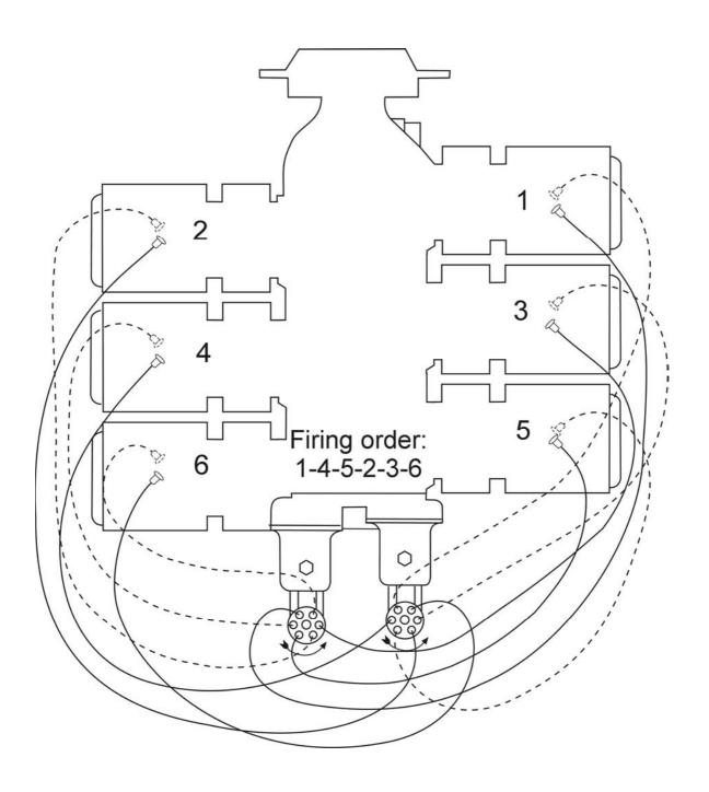
Figure 5-3. Ignition Wiring Diagram – Dual Magneto
