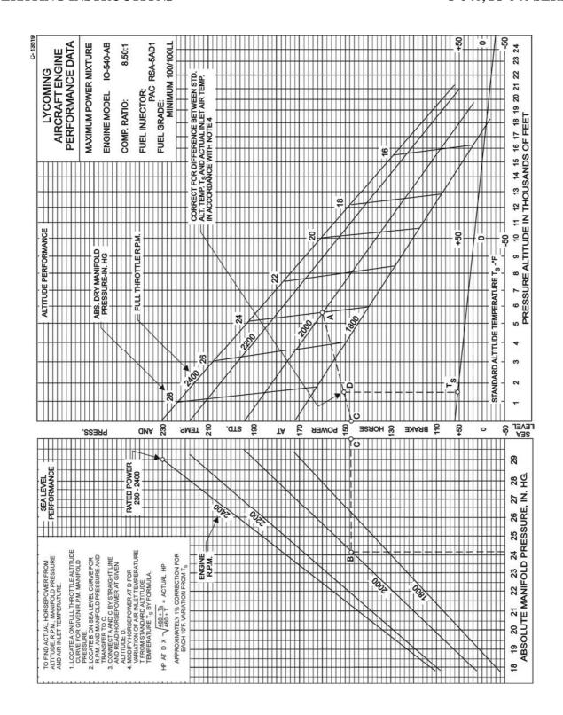
Figure 3-28. Sea Level and Altitude Performance Curve – IO-540-AB Series
