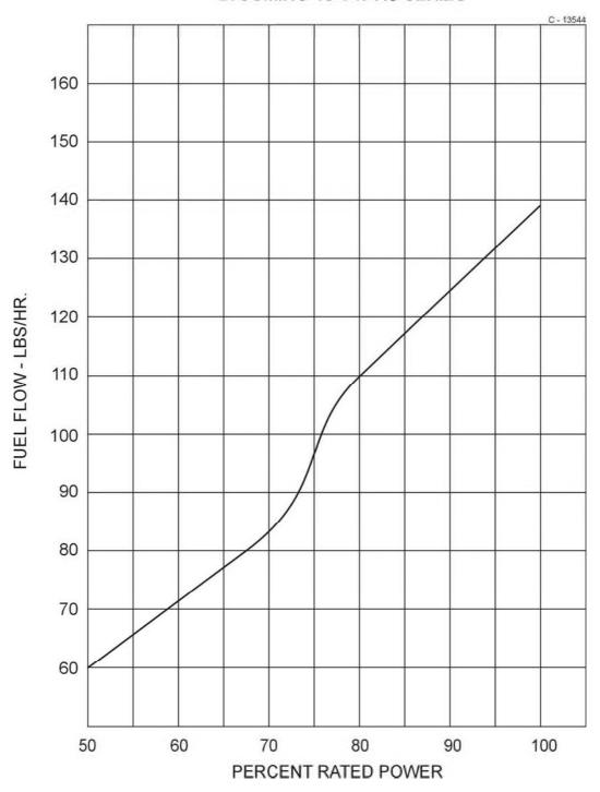
Figure 3-29. Fuel Flow vs Percent Rated Power – IO-540-AC Series
