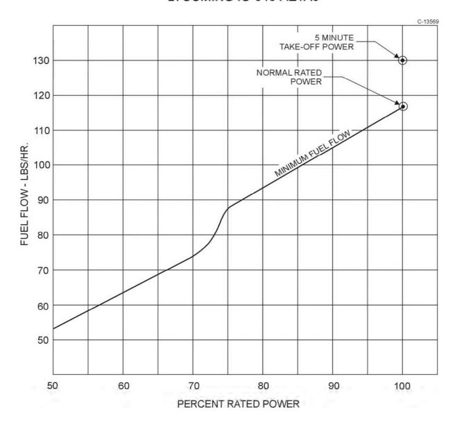
Figure 3-30. Fuel Flow vs Percent Rated Power – IO-540-AE Series
