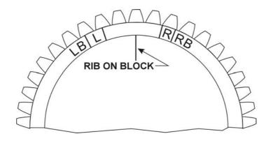
Figure 5-2. Timing Marks – 6 Cylinder –1200 Series
