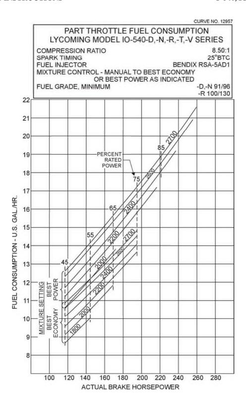
Figure 3-18. Part Throttle Fuel Consumption Curve – IO-540-D, -N, -R, -T, -V
