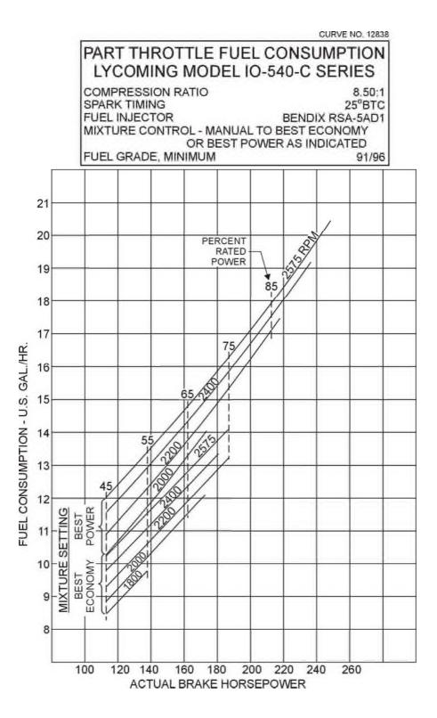
Figure 3-16. Part Throttle Fuel Consumption Curve – IO-540-C
