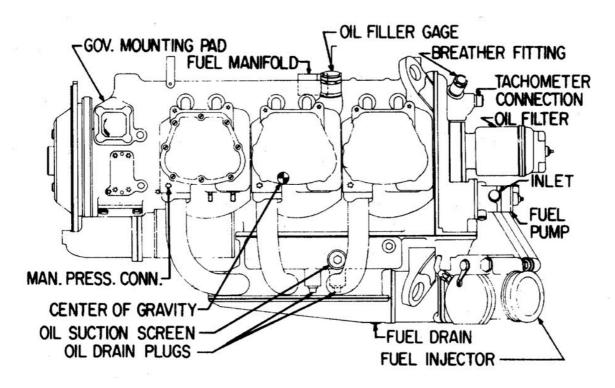
Figure 7-9. Installation Drawing – Left Side View – IO-540-K
