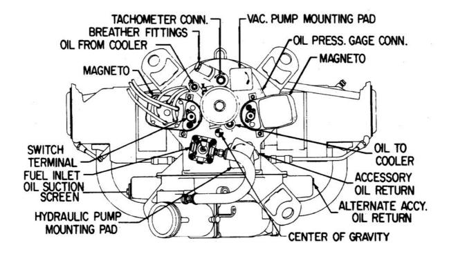
Figure 7-10. Installation Drawing – Rear View – IO-540-K
