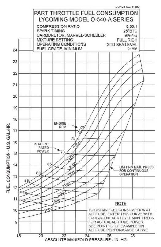
Figure 3-2. Part Throttle Fuel Consumption Curve – O-540-A
