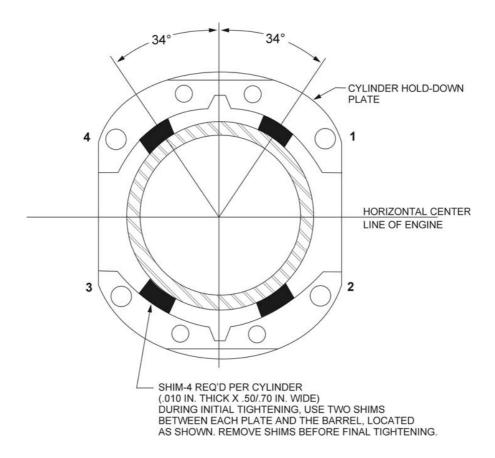
Figure 5-4. Location of Shims Between Cylinder Barrel and Hold-Down Plates (where applicable) and Sequence of Tightening Cylinder Base Hold-Down Nuts
