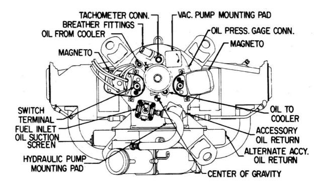
Figure 7-2. Installation Drawing – Rear View – O-540 Series
