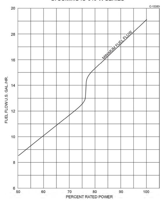
Figure 3-24. Fuel Flow vs Percent Rated Power Curve – IO-540-W Series
