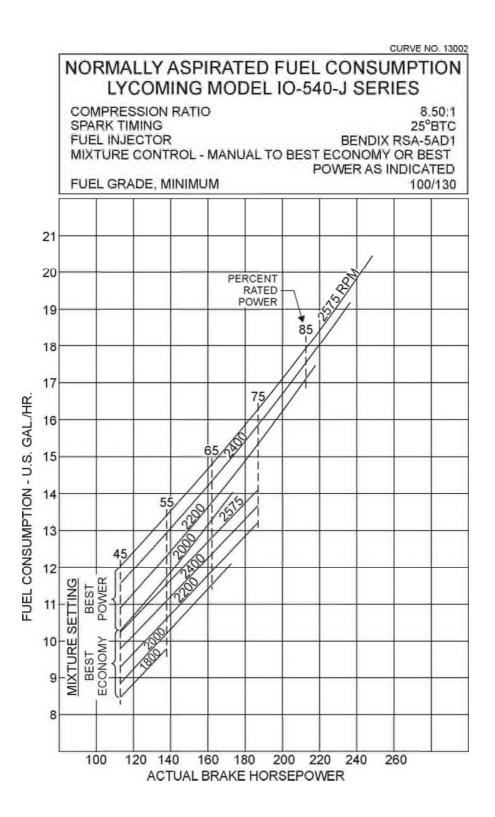
Figure 3-20. Normally Aspirated Fuel Consumption Curve – IO-540-J
