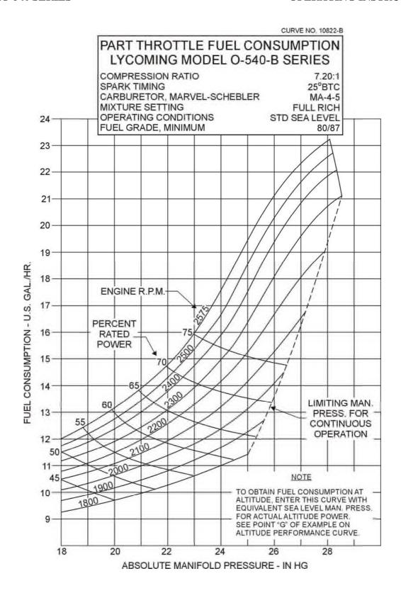
Figure 3-5. Part Throttle Fuel Consumption Curve – O-540-B
