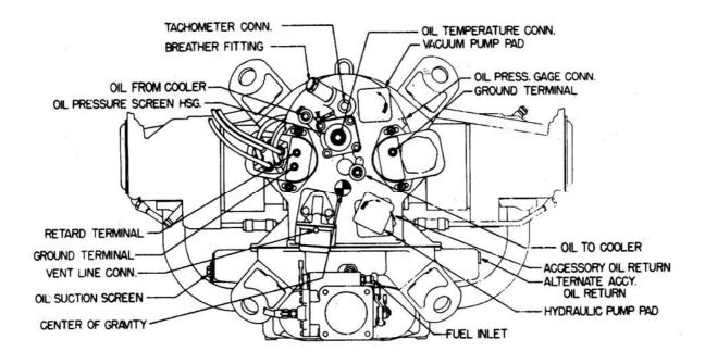
Figure 7-6. Installation Drawing – Rear View – IO-540-B, -E
