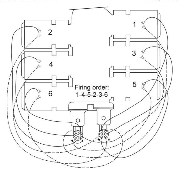
Figure 5-1. Ignition Wiring Diagram
