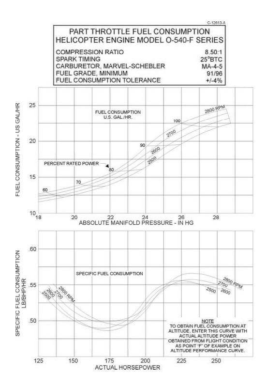
Figure 3-10. Part Throttle Fuel Consumption Curve – O-540-F Series
