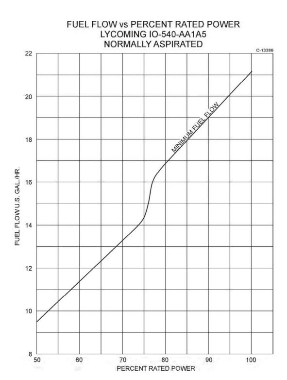
Figure 3-26. Fuel Flow vs Percent Rated Power – IO-540-AA1A5
