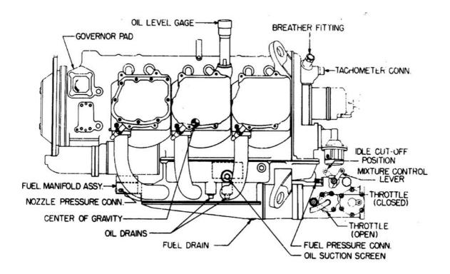
Figure 7-5. Installation Drawing – Left Side View – IO-540-B, -E
