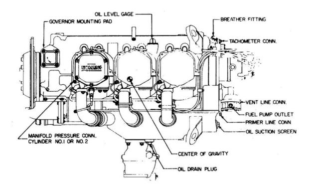
Figure 7-1. Installation Drawing – Left Side View – O-540 Series
